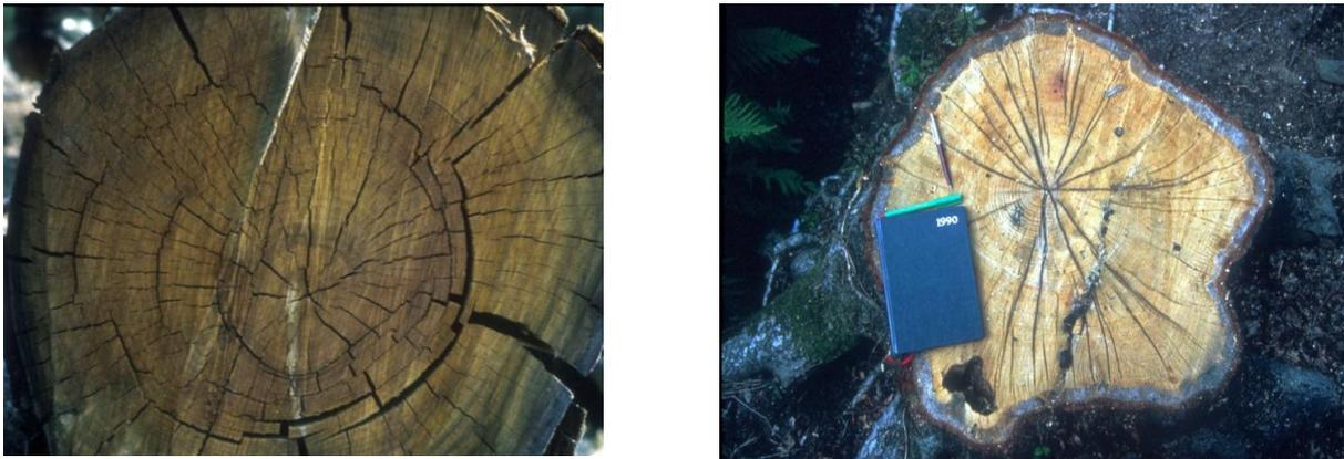
Figure 1. Shaken logs of oak. Left, ring shake, right star shake
