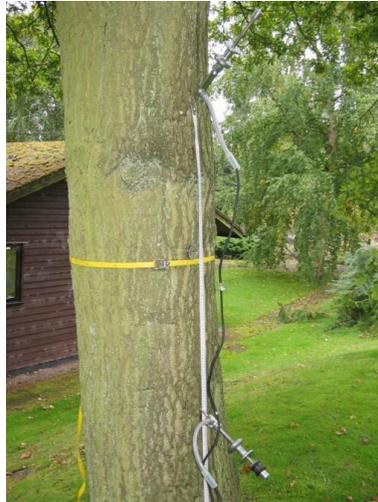
Figure 3. Acoustic tool in use. The picture shows the probes only: the meter that measures the time is out-of-shot.
