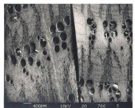
Figure 2. Horizontal sections of oak timber showing a tree with very large early wood vessels (left) and smaller vessels (right)
