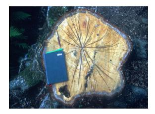
Figure 1. Shaken logs of oak. Left, ring shake, right star shake
