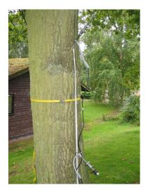
Figure 3. Acoustic tool in use. The picture shows the probes only: the meter that measures the time is out-of-shot.
